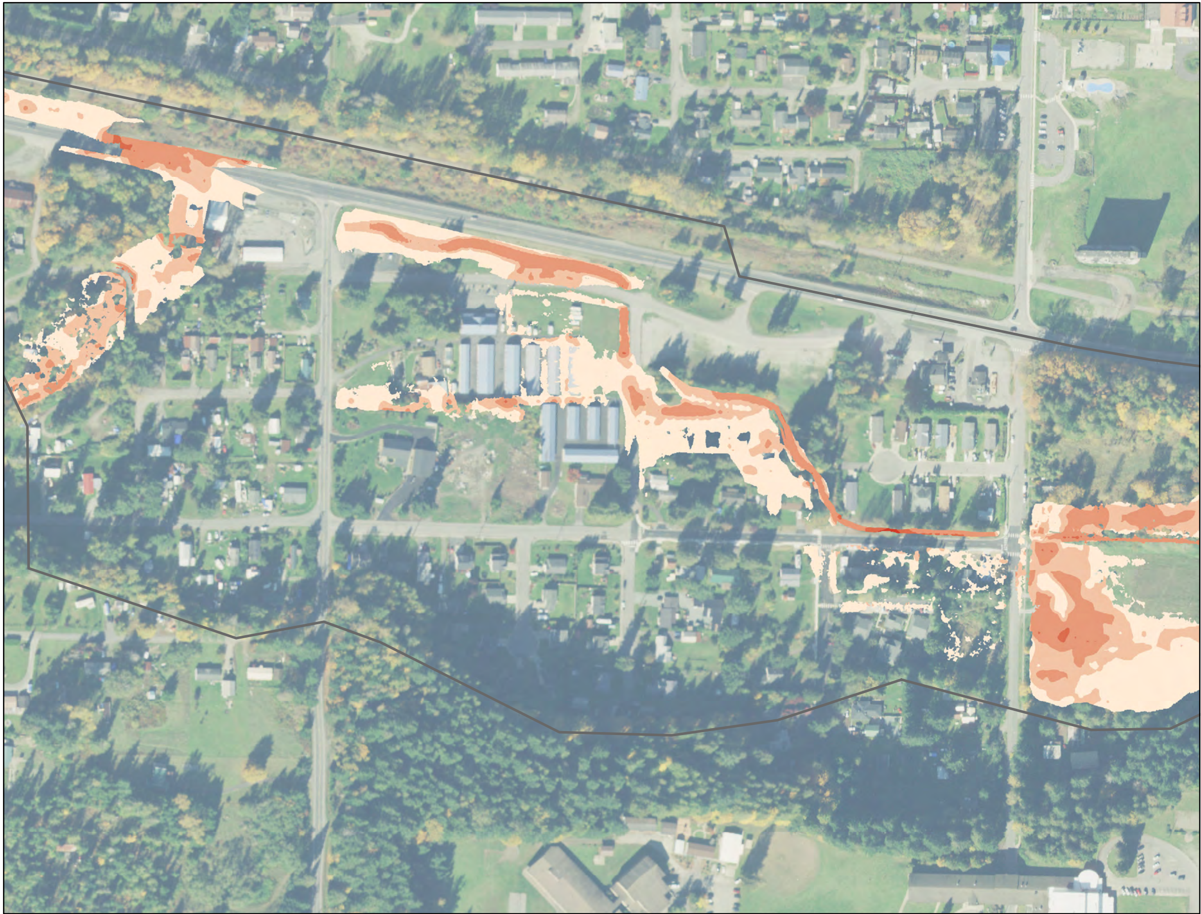
Figure 6. Lorenzan Creek Hydraulic Model Results Existing Conditions
