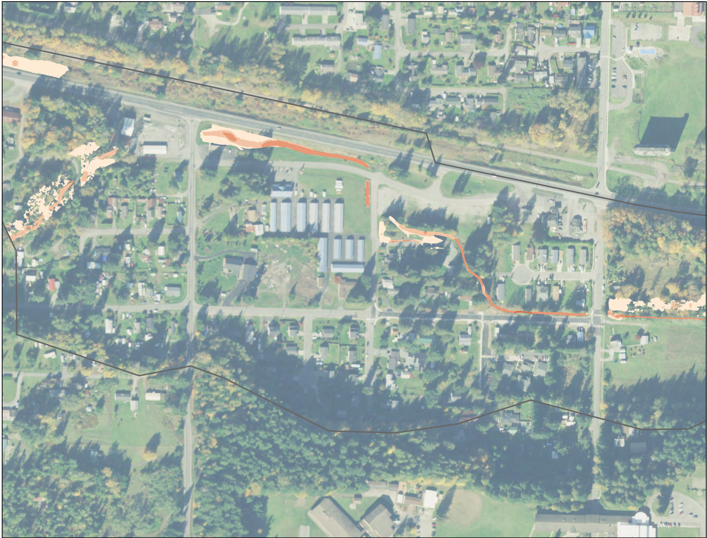
Figure 4. Lorenzan Creek Hydraulic Model Results Existing Conditions
