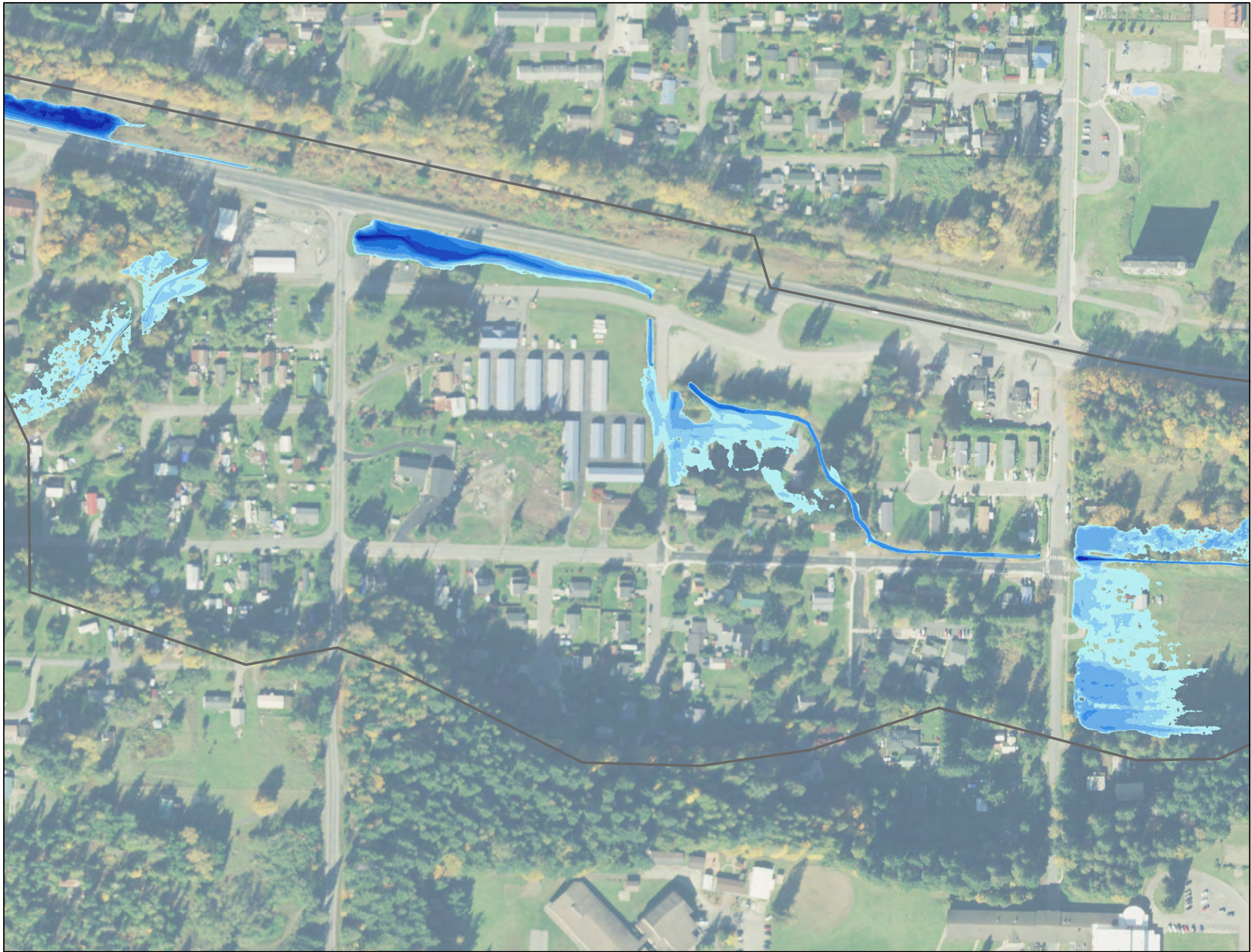
Figure 2. Lorenzan Creek Hydraulic Model Results Existing Conditions
