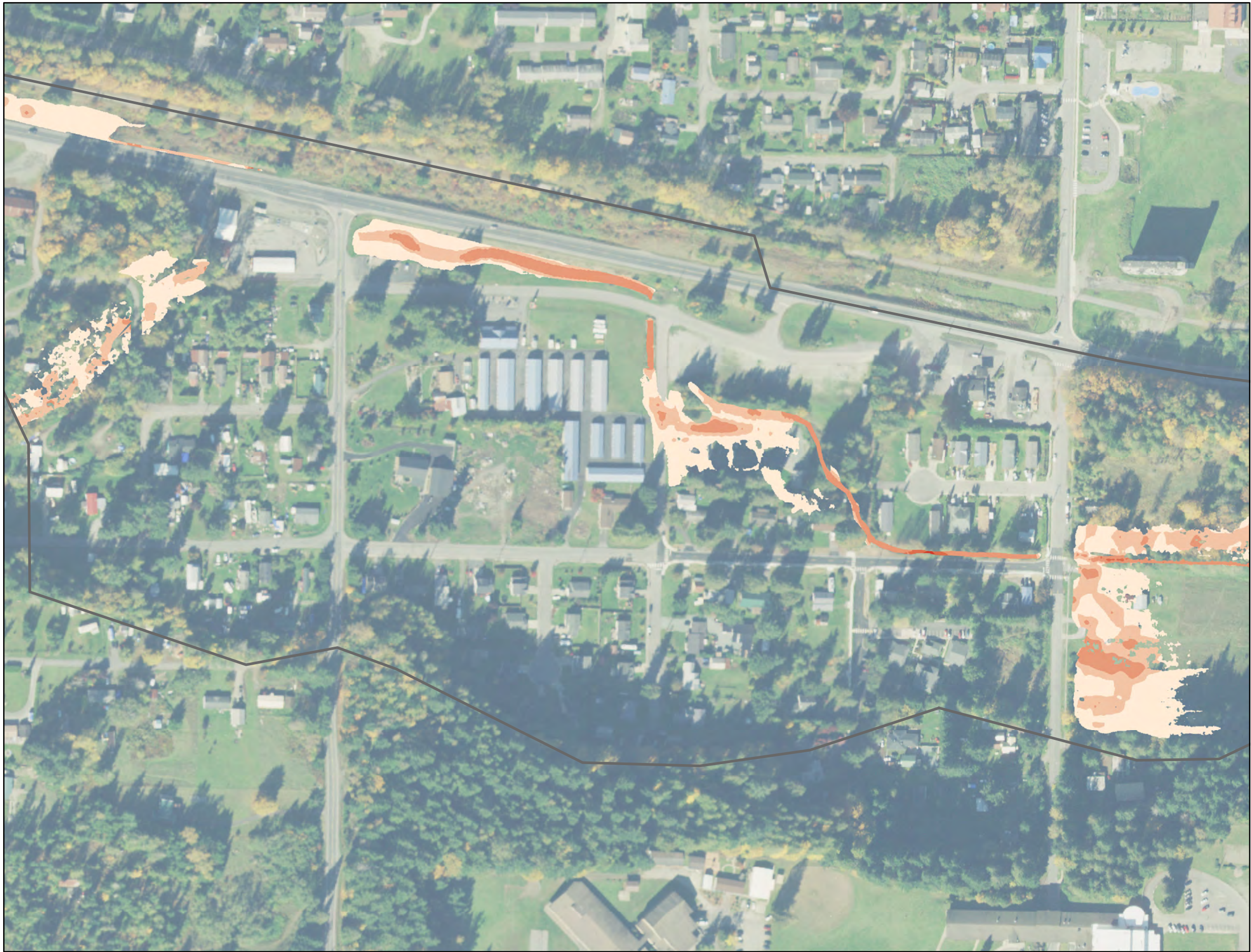
Figure 5. Lorenzan Creek Hydraulic Model Results Existing Conditions
